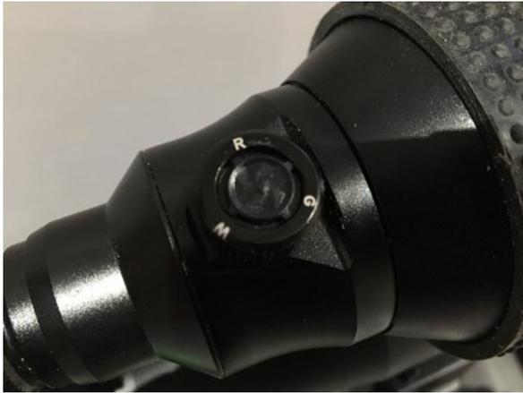
**ABOVE:** The three colours can be accessed by a simple dial on the top of the torch
